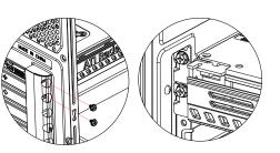
Remove the PCI slot protection cover. Install the graphics card and secure it with a screw.
